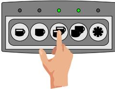
When you have powered up the machine you will see that the LED's on both buttons 3 and 4 now light up. If they do not light up please recheck that you have the jumpers in the correct locations. Once you see both LED's light up you can remove your finger from the keypad.
