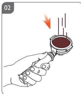
▲ Fill the filter basket of the porta-filter with espresso powder (the amount may differ depending of the filter basket size). For best result use freshly ground espresso beans.
