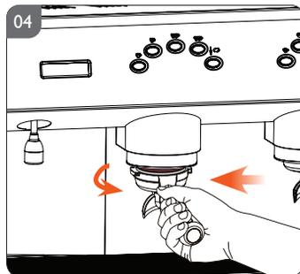
▲ Insert the filled porta-filter into the group head and lock it into correct position.
