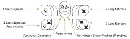
The Continuous Dispensing button performs 3 different functions (depending on length of time pressed):
