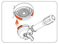
Align the porta-filter's two lateral flanges with the slots in the group.
