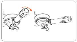
Insert the porta-filter and rotate it anti-clockwise until the handle is perpendicular to the coffee machine.
