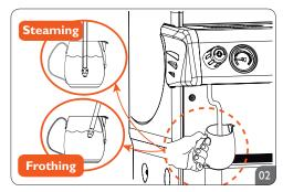
Immerse the steam wand into the jug containing the milk, make sure the wand tip is submerged.
