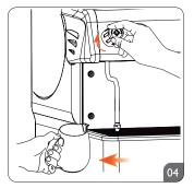
Once the milk reaches the desired temperature, close the tap and remove the jug.
